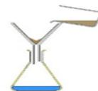
Separates an **insoluble solid** from a **mixture**. E.g. **sand** from **water**.
